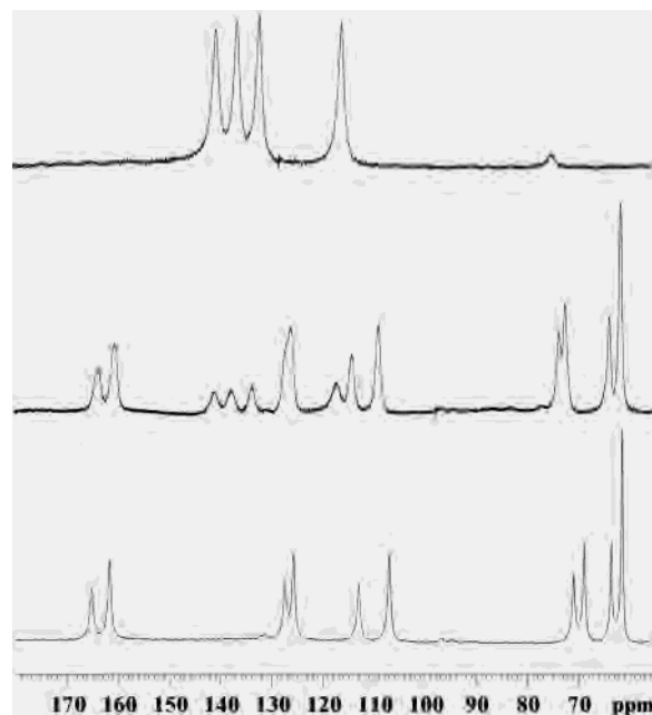
Figure 5. Low-field portion of the 1 H NMR spectra of an aqueous solution of [Yb(BrBzDO3A)] free (top) and upon addition of ( S )-lactate with a molar ratio of 0.9:1 (middle) and 10:1 (bottom) (7.05 T; pH 6.5; 298 K).
