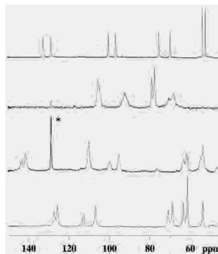
Figure 8. Low-field portion of the ^1\text{H} NMR spectra at 298 K and pH 6.5 of the ternary adduct with ( S )-lactate of the following (from top to bottom): [\text{Yb}(\text{MBzDO3AM})]^{3+} , [\text{Yb}(\text{DO3A})] , [\text{Yb}(\text{MBzDO3A})] , and [\text{Yb}(\text{BrBzDO3A})] . The signal labeled with an asterisk refers to the presence of [\text{Yb}(\text{DOTA})]^- as impurity.
